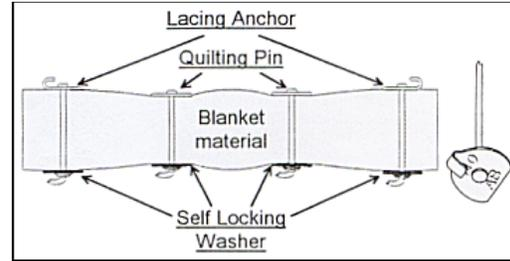
**GEMCO lacing anchors and quilting pins are used in the manufacture of removeable blanket insulation.**
