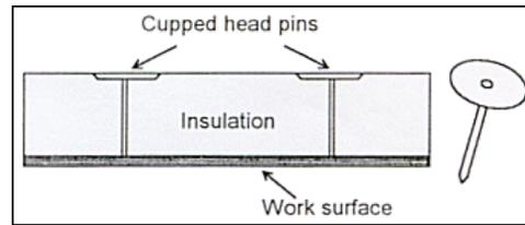
**GEMCO cupped head pins are welded directly through insulation.**
