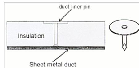
**GEMCO duct liner pins are used in the HVAC industry.**
